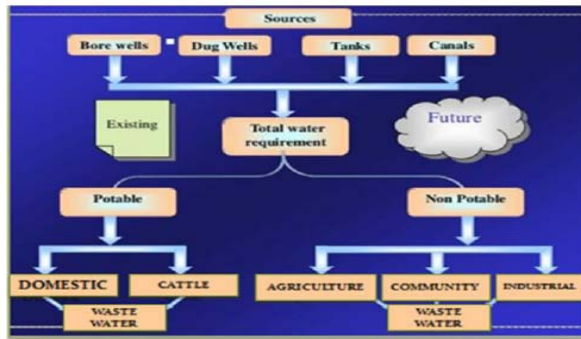
Fig. 1 Traditional approach of water supply
